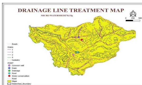
Figure 9 – Drainage line treatment map
