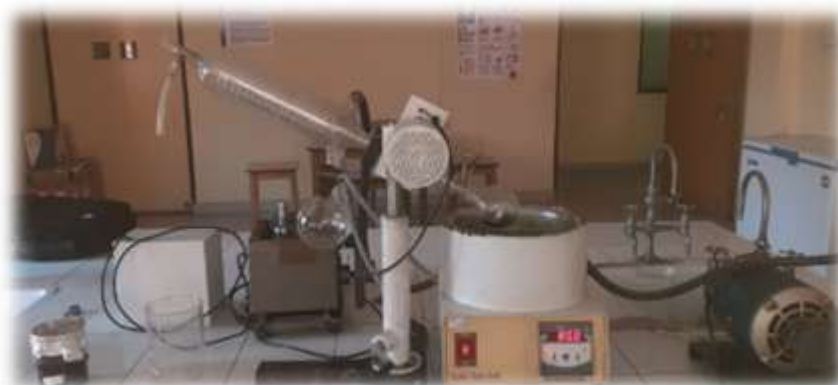
Fig. 6. Two-stage evaporation of filtered extract through digital water bath for concentration, with primary evaporation at 80°C for 3 hours to preserve thermolabile alkaloids.
