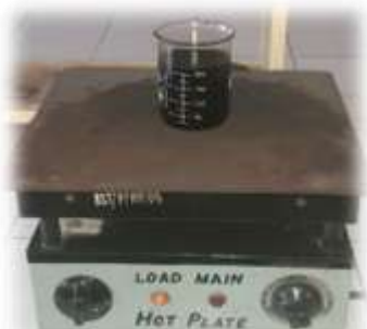
Fig. 7. Reduced-temperature evaporation through hot pate for secondary concentration to prevent thermal decomposition
