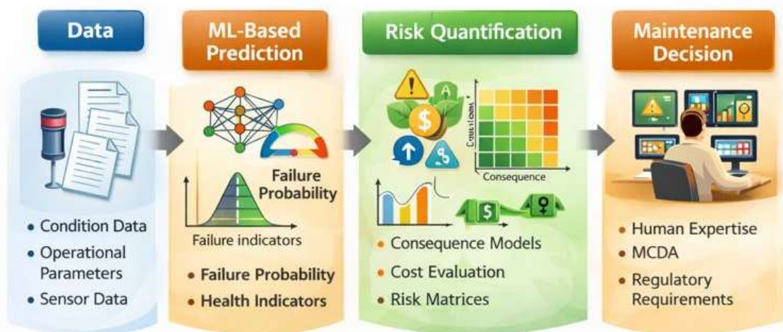
Figure 2. ML-Enabled Risk-Based Maintenance Decision Pipeline
