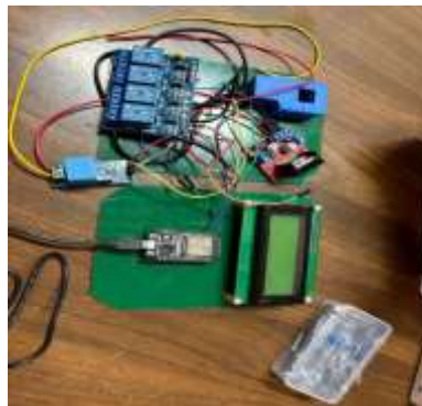
Fig. 6: Proof of Concept Hardware Model of Smart Energy Monitoring System
